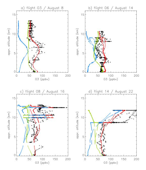
Fig. 1. Vertical profiles of observed ozone (black), modeled ozone (red) and contributions by  $O_{3s}$  (blue) and  $O_{3t}$  (green) for several MINOS flights.
