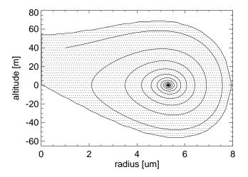
**Fig. 3.** Stability region of UTTCs. The ice particles starting within the stability region (given by initial size and altitude) survive and spiral to the equilibrium size and altitude. Particles outside this region evaporate at the lower altitude with  $S_{\rm ice} < 1$ . Trajectory refers to an ice particle with  $r = 1 \, \mu \rm m$  released 40 m above the equilibrium position. The altitude given here is relative to the equilibrium position of the UTTCs.
