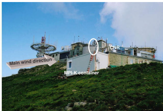
Fig. 2. A measuring container housing the CIMS instrument was set up upwind from the CNR station with respect to the main wind direction (prevailing winds blow from SW) as indicated. In this way ambient air was sampled approximately 4.5 m above the ground and about 1 m above and in front of the container. The inlet pointed outwards towards the edge of the southern mountainside of Monte Cimone, i.e. in the main wind direction.
