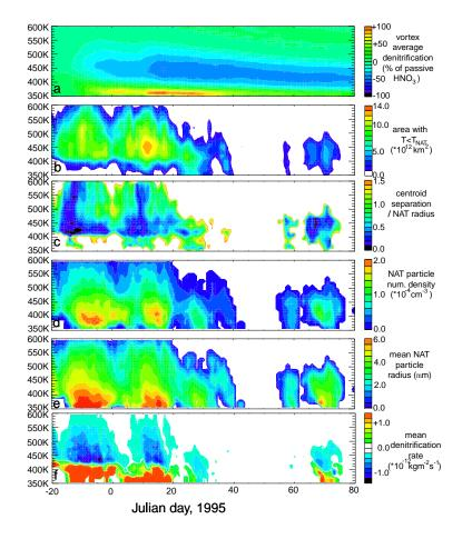
**Fig. 3.** Altitude time plots for winter 1994/95 of (**a**) vortex average denitrification; (**b**) area of Arctic stratosphere below  $T_{\text{NAT}}$ ; (**c**) normalized centroid separation; (**d**) particle number concentration; (**e**) mean particle radius; and (**f**) denitrification rate.
