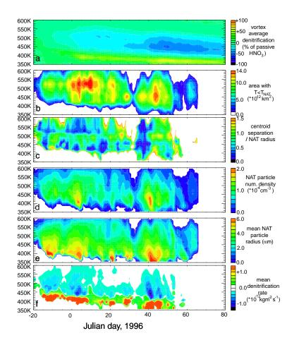
**Fig. 4.** Altitude time plots for winter 1995/96 of (**a**) vortex average denitrification; (**b**) area of Arctic stratosphere below  $T_{\text{NAT}}$ ; (**c**) normalized centroid separation; (**d**) particle number concentration; (**e**) mean particle radius; and (**f**) denitrification rate.
