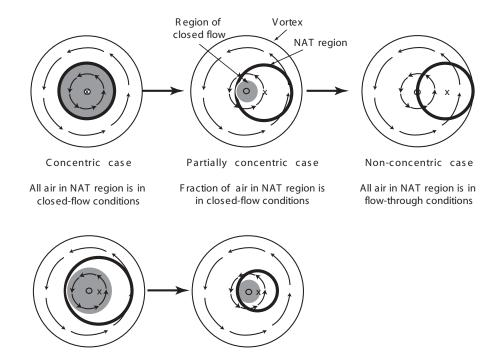
**Fig. 8.** Schematic of how the NAT area-vortex centroid separation and the NAT area area control the denitrification rate. The "closed-flow" region is shaded. (a) The effect of shifting the NAT area away from the centre of the vortex; (b) the effect of reducing the size of the NAT area.
