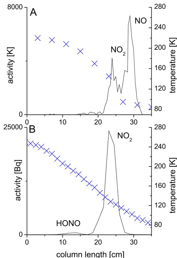
**Fig. 5.** Comparison of two chromatograms with different experimental conditions. The activity is given on the left axis (solid line) and the temperature along the column at the right axis (crosses). In experiment A the temperature was always too low for a quasi-liquid layer to form, whereas in chromatogram B a quasi liquid layer might have evolved. Note that the two NO<sub>2</sub> peaks should be compared; the NO in experiment A was added on purpose, without any relation to this comparison.
