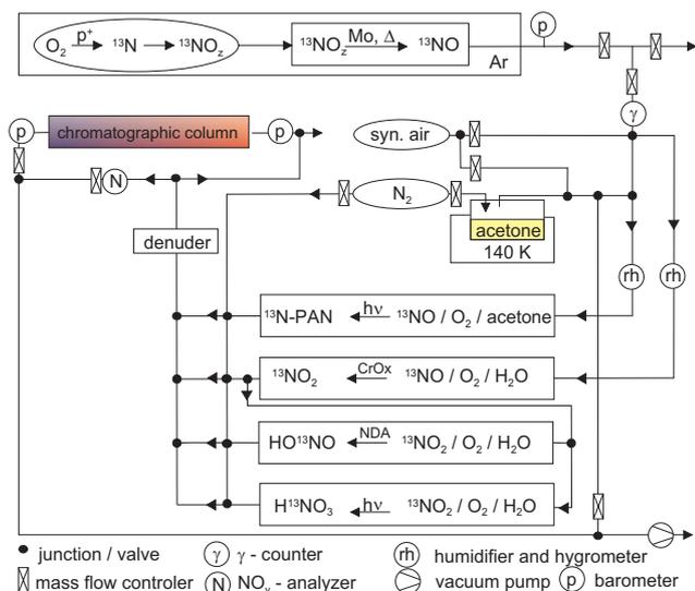
**Fig. 1.** Experimental set-up: gas target to produce <sup>13</sup>N, photolysis cells to oxidize the nitrogen oxides and chromatographic column.
