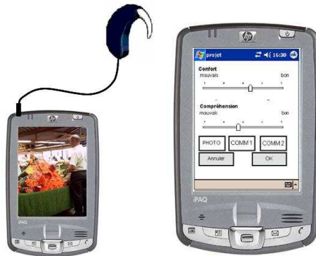
Fig. 11. A sampling software has been developed on a PDA that the patient plugs directly onto the CI processor in order to sample the exact sound that is received by the processor.
