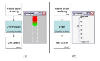
Figure 7: Two graphical modalities based on a mini-screen but with different interaction languages: (a) a colour gauge; (b) a slider.
