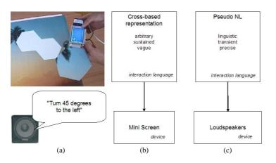
Figure 2: Examples of ICARE elementary components developed for a puzzle game. (a) A puzzle piece with a mini-screen that displays guidance information as two crosses, one mobile (the current orientation) and one static (the right orientation) (M1), while playing a pseudo natural language oral message (M2); (b) ICARE components for modality M1 = <cross-based graphical representation, mini-screen>; (c) ICARE components for modality M2 = seudo NL, loudspeakers>.
