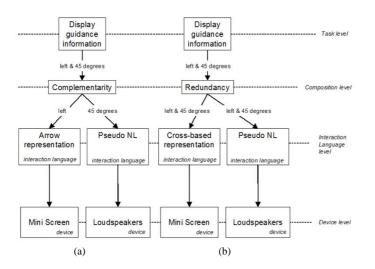
**Figure 4:** Examples of ICARE combination components developed for a puzzle game. (a) Two complementary modalities. (b) Two redundant modalities.
