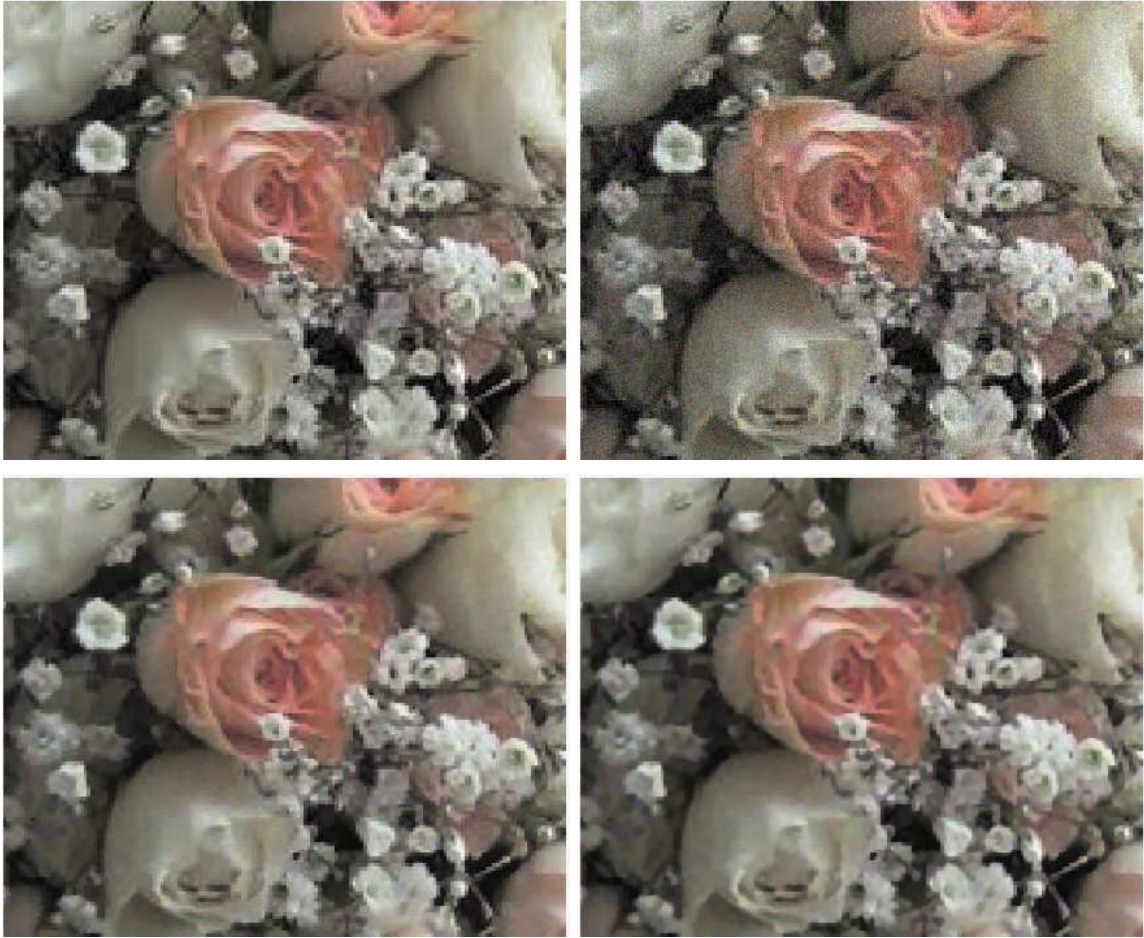
Figure 2: First row: original and noisy images (PSNR = 56.9 dB). Second row: denoised with color ROF ( \lambda = 15 , PSNR= 73.8 dB) and with color OSV ( \lambda = 15 , PSNR= 73.4 dB).
