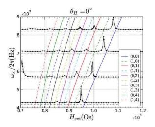
FIG. 12: (Color online) Comparison between the 2D analytical model (oblique lines) and the 3D micromagnetic simulation (horizontal spectra) for the prediction of the resonance fields of a  $D_2 = 0.5 \ \mu m$  Py disk magnetized at  $\theta_H = 0^\circ$ . The continuous lines are the locus of the resonance field of the radial modes ( $\ell = 0, m$ ) predicted analytically (dashed lines correspond to the hidden modes ( $\ell = 1, m$ )).
