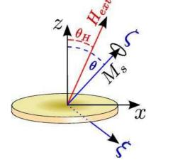
FIG. 11: (Color online) Graphic representation of the Cartesian frame  $(\xi, \zeta)$  (blue) rotated in the direction of the equilibrium magnetization, when the applied field makes an angle  $\theta_H$  with the normal of the disk (z-axis).
