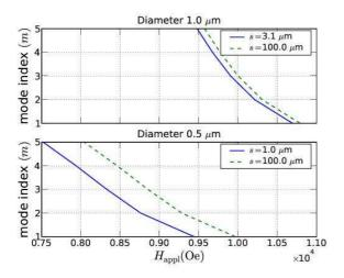
FIG. 7: (Color online) Calculated spectral deformation induced by the magnetic tip placed at distances s = 3.1 and 1.0  $\mu$ m above the disk samples  $D_1 = 1.0$  and  $D_2 = 0.5 \mu$ m, respectively. The graphs show the downward shift in field of each resonance mode (indexed by m) compared to the unperturbed FMR spectrum (dashed line).
