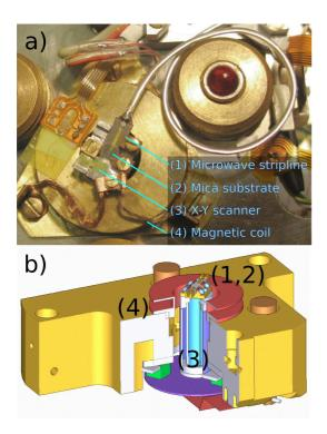
FIG. 2: (Color online) a) Photography of the MRFM bottom base showing (1) the microwave antenna, (2) the mica substrate where the Py disks are, (3) the piezo-electric scanner, and (4) the magnetic coil used for a calibrated modulation of the applied field. b) Section view of the above elements. The top part with the cantilever and the optical detection is not shown.
