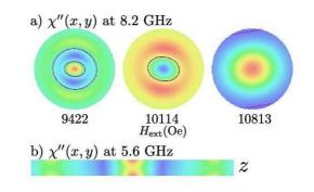
FIG. 13: (Color online) a) Images of the transverse susceptibility obtained through the 3D micromagnetic simulation for the first three modes at 8.2 GHz of a  $D_2 = 0.5 \ \mu m$  Py disk magnetized at  $\theta_H = 0^\circ$ . The thick lines indicate the nodes of precession. b) Image of the transverse susceptibility for the third mode (at  $H_{\rm ext} = 8.8$  kOe) of the 5.6 GHz spectrum showing that the magnetization dynamics is not uniform across the thickness of the disk.
