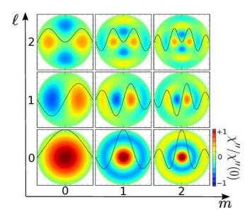
FIG. 6: (Color online) Color code representation of the eigenmodes basis  $\mathcal{J}_m^\ell(\mathbf{r})$ , where  $\ell$  and m indicate respectively the number of nodes in the circumferential and radial direction. Only the modes  $\ell = 0$  couple to a uniform microwave excitation.
