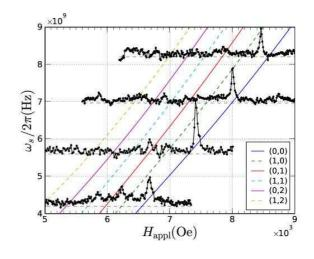
FIG. 10: (Color online) Mechanical-FMR spectra of the  $D_2 = 0.5 \ \mu \text{m}$  disk measured at 4.2, 5.6, 7.0 and 8.2 GHz and  $s \approx 1.0 \ \mu \text{m}$ . The lines are the analytical predictions of the locus of the  $(\ell, m)$ -modes when  $\theta_H = 9.5^\circ$  and  $H_{\text{off}} = -760$  Oe.
