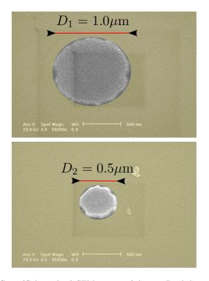
FIG. 8: (Color online) SEM images of the two Py disks samples. The images are being viewed at an angle, thus distorsions exist in the vertical direction.
