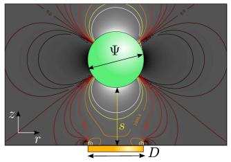
FIG. 3: (Color online) Visualization of the dipolar coupling interaction between a spherical magnetic probe (diameter  $\Psi$ ) and a cylindrical Py disk (diameter D) separated by a distance s. The magnetic configurations in both objects are assumed to be saturated along z. The color lines represent the iso- $B_z$ field lines. The bright and dark shades separate respectively the positive and negative coupling regions.
