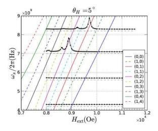
FIG. 14: (Color online) Comparison between the 2D analytical model (oblique lines) and the 3D micromagnetic simulation (horizontal spectra) for the prediction of the resonance fields of a  $D_2 = 0.5 \ \mu m$  Py disk magnetized at  $\theta_H = 5^\circ$ . The continuous lines are the locus of the resonance field of the radial modes ( $\ell = 0, m$ ) predicted analytically (dashed lines correspond to the hidden modes ( $\ell = 1, m$ )).
