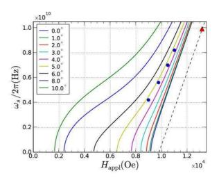
FIG. 16: (Color online) Resonance field (blue dots) of the fundamental mode measured on the  $D_1 = 1.0 \ \mu \text{m}$  disk along with the analytically predicted angle dependence of  $H_{\text{res}}(\omega_s)$  for different values of  $\theta_H$  (lines). Also indicated is the measured resonance position in the extended film (red triangle) and the gyromagnetic ratio (dashed line): the shift with the  $\theta_H = 0^\circ$  line is due to finite size effects in the disk.
