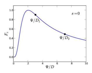
FIG. 4: (Color online) Variation of the dipolar magnetic force between a sphere and a disk in contact (s = 0) as a function of the ratio between their diameters, respectively  $\Psi$  and D. The maximum force occurs when  $\Psi = 2D$ .
