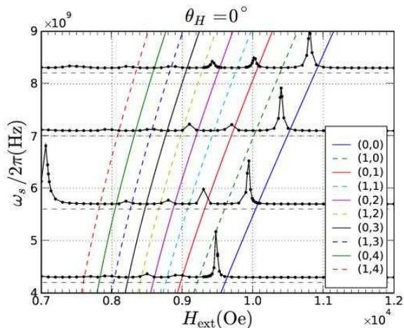
FIG. 12: (Color online) Comparison between the 2D analytical model (oblique lines) and the 3D micromagnetic simulation (horizontal spectra) for the prediction of the resonance fields of a  $D_2 = 0.5 \mu\text{m}$  Py disk magnetized at  $\theta_H = 0^\circ$ . The continuous lines are the locus of the resonance field of the radial modes ( $\ell = 0, m$ ) predicted analytically (dashed lines correspond to the hidden modes ( $\ell = 1, m$ )).
