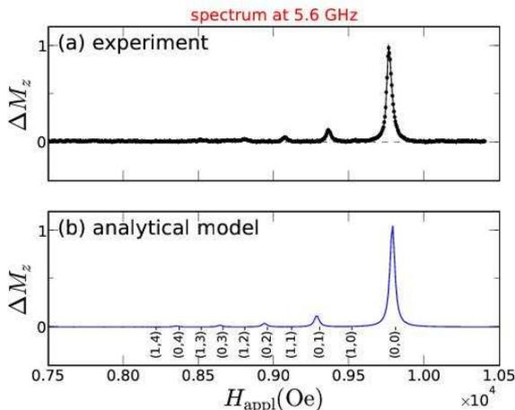
FIG. 17: (Color online) Comparison between experiment and analytical model of the amplitude of the peaks for the disk of diameter  $1.0 \mu\text{m}$  at  $5.6 \text{ GHz}$ .
