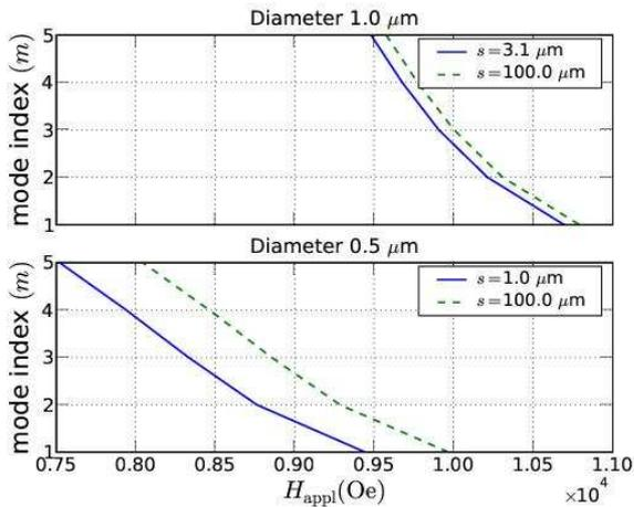
FIG. 7: (Color online) Calculated spectral deformation induced by the magnetic tip placed at distances  $s = 3.1$  and  $1.0 \mu\text{m}$  above the disk samples  $D_1 = 1.0$  and  $D_2 = 0.5 \mu\text{m}$ , respectively. The graphs show the downward shift in field of each resonance mode (indexed by  $m$ ) compared to the unperturbed FMR spectrum (dashed line).
