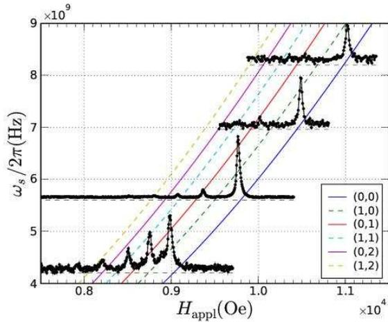
FIG. 9: (Color online) Mechanical-FMR spectra of the  $D_1 = 1.0 \mu\text{m}$  disk measured at 4.2, 5.6, 7.0 and 8.2 GHz and  $s \approx 3.1 \mu\text{m}$ . The lines are the analytical predictions of the locus of the  $(\ell, m)$ -modes when  $\theta_H = 4.9^\circ$  and  $H_{\text{off}} = -70 \text{ Oe}$ .
