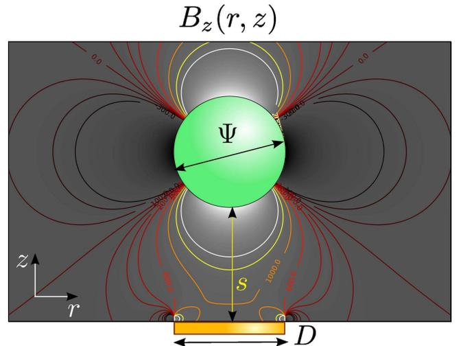
FIG. 3: (Color online) Visualization of the dipolar coupling interaction between a spherical magnetic probe (diameter  $\Psi$ ) and a cylindrical Py disk (diameter  $D$ ) separated by a distance  $s$ . The magnetic configurations in both objects are assumed to be saturated along  $z$ . The color lines represent the iso- $B_z$  field lines. The bright and dark shades separate respectively the positive and negative coupling regions.
