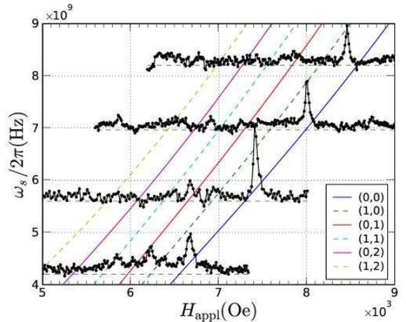
FIG. 10: (Color online) Mechanical-FMR spectra of the  $D_2 = 0.5 \mu\text{m}$  disk measured at 4.2, 5.6, 7.0 and 8.2 GHz and  $s \approx 1.0 \mu\text{m}$ . The lines are the analytical predictions of the locus of the  $(\ell, m)$ -modes when  $\theta_H = 9.5^\circ$  and  $H_{\text{off}} = -760 \text{ Oe}$ .
