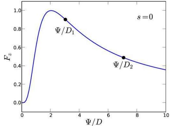
FIG. 4: (Color online) Variation of the dipolar magnetic force between a sphere and a disk in contact ( $s = 0$ ) as a function of the ratio between their diameters, respectively  $\Psi$  and  $D$ . The maximum force occurs when  $\Psi = 2D$ .
