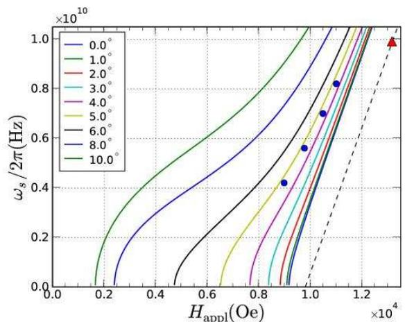
FIG. 16: (Color online) Resonance field (blue dots) of the fundamental mode measured on the  $D_1 = 1.0 \mu\text{m}$  disk along with the analytically predicted angle dependence of  $H_{\text{res}}(\omega_s)$  for different values of  $\theta_H$  (lines). Also indicated is the measured resonance position in the extended film (red triangle) and the gyromagnetic ratio (dashed line): the shift with the  $\theta_H = 0^\circ$  line is due to finite size effects in the disk.
