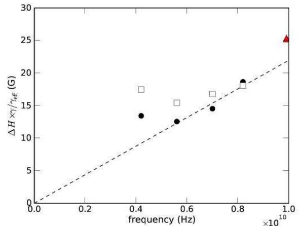
FIG. 18: (Color online) Frequency dependence of the line width measured on both the  $D_1 = 1.0 \mu\text{m}$  disk (full circles) and the  $D_2 = 0.5 \mu\text{m}$  disk (open boxes). The red triangle indicates the value measured by cavity-FMR on the extended film on Si. The mechanical-FMR data are renormalized by  $\gamma_{\text{eff}}$ . The dashed line corresponds to a damping coefficient  $\alpha = 6 \times 10^{-3}$ .
