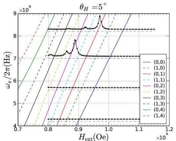
FIG. 14: (Color online) Comparison between the 2D analytical model (oblique lines) and the 3D micromagnetic simulation (horizontal spectra) for the prediction of the resonance fields of a  $D_2 = 0.5 \mu\text{m}$  Py disk magnetized at  $\theta_H = 5^\circ$ . The continuous lines are the locus of the resonance field of the radial modes ( $\ell = 0, m$ ) predicted analytically (dashed lines correspond to the hidden modes ( $\ell = 1, m$ )).
