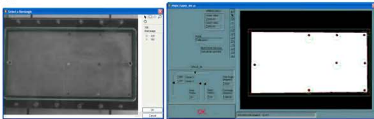
FIGURE 4. Selection of region of interest (left) and detection of gate inlet and vacuum outlets
