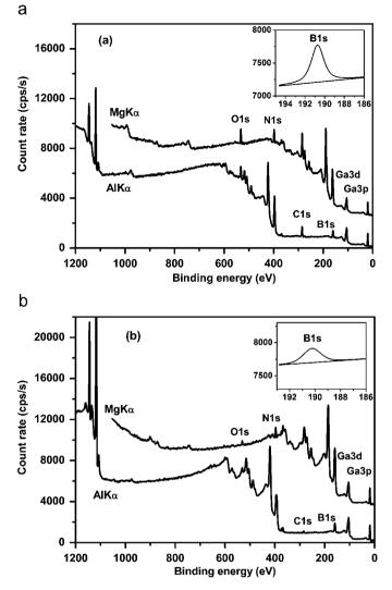
**Fig. 5.** Typical XPS spectra of BGaN film deposited for TEB/III ratio of 6% (a) before and (b) after surface sputtering. The insets compare the boron peaks evolution with sputtering.
