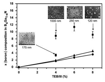
**Fig. 6.**  $B_xGa_{1-x}N$  boron composition (%) versus TEB/III ratio deduced from XPS measurements before (squares) and after sputtering (triangles). Error bars represent the accuracy of the method ( $\pm 10\%$ ). XRD data are shown with circles. The insets present BGaN surface morphology before sputtering.
