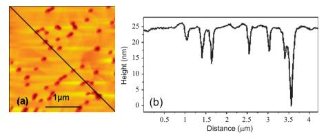
Fig. 2. (a) 3 × 3 µm<sup>2</sup> surface AFM image and (b) cross-sectional scan of GaN buffer layer. The solid line on the 2D AFM image corresponds to the cross-sectional scan.
