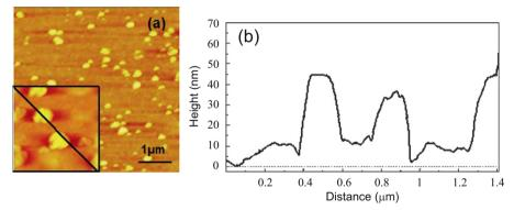
**Fig. 4.** The  $5 \times 5 \,\mu\text{m}^2$  and  $1 \times 1 \,\mu\text{m}^2$  (inset) 2D AFM topography and corresponding cross-sectional scan of 170 nm thick BGaN epilayer grown at the TEB/III ratio of 6%. The solid line on the 2D AFM image corresponds to the cross-sectional scan.
