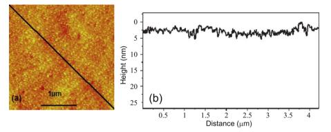
**Fig. 3.** (a)  $3 \times 3 \mu m^2$  surface AFM image and (b) cross-sectional scan of 50 nm thick  $B_{0.027}Ga_{0.073}N$  film. The solid line on the 2D AFM image corresponds to the cross-sectional scan.
