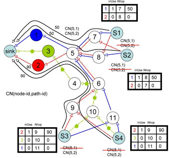
Fig. 2. Initial configuration, then congestion notification from node 5.
