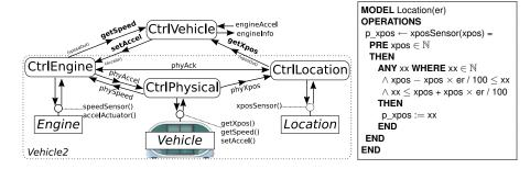
Fig. 9. The Vehicle2 component
