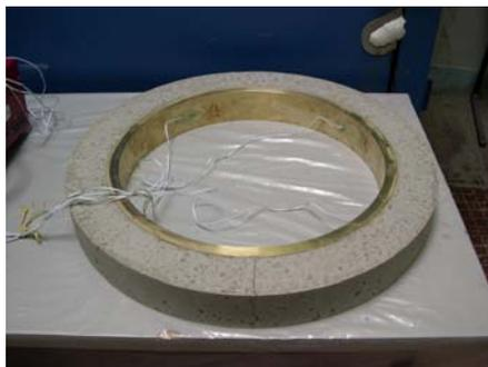
**Figure 3.** The ring test
