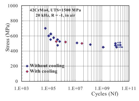
**Fig. 10** Fatigue test results of 42CD4 (20 kHz, R = -1 in air).
