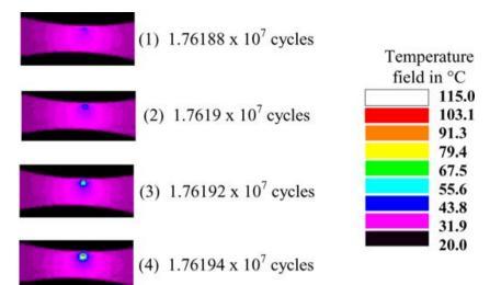
Fig. 9 Temperature field just before rupture; 42CD4 steel with stress amplitude of 425 MPa; test 5.
