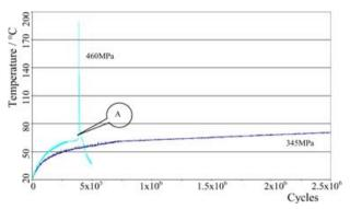
Fig. 7 Temperature profiles of 42CD4 tested at different stress level (f = 20 kHz); tests 5 and 6.
