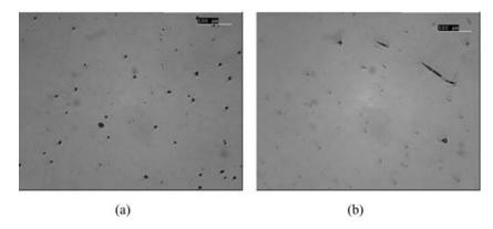
Fig. 1 Optical micrographs (a) AISI 52100 microstructure with small inclusion. (b) 42CD4 microstructure with MnS inclusion.
