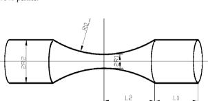
Fig. 3 Geometry of specimen.
