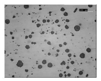
**Fig. 2** Optical micrographs of cast iron GS51 with 5% ferrite and 95% perlite.
