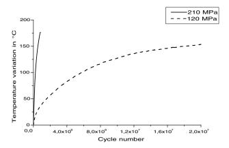
Fig. 5 Temperature variation at the centre of the specimen; cast iron GS51; tests 3 and 4.
