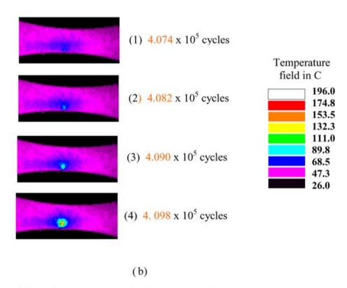
Fig. 8 Temperature field just before rupture; 42CD4 steel with stress amplitude of 460 MPa; test 6.
