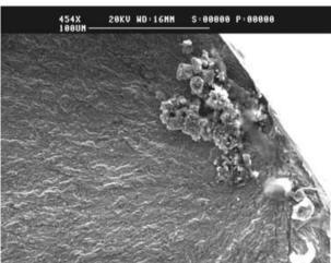
Fig. 12 Fracture surface due to non-metallic inclusions (under jacket) in microstructure of 42CD4 T (R=-1, 20 kHz,  $N_{\rm f}=7.1\times10^7$  cycles).
