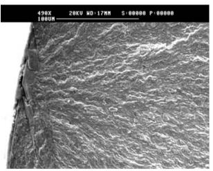
Fig. 11 Fracture surfaces due to non-metallic inclusions (at the surface) in microstructure of 42CD4 T (R=-1, 20 kHz,  $N_{\rm f}=1\times10^6$  cycles).
