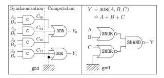
Figure 1: Schematic of the QDI secured AND gate (*left*) and its internal 30R architecture (*right*).
