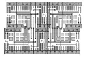
Figure 7: SecLib two-input AND gate floorplan (top), structure (middle) and interface (bottom.)
