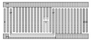
Figure 5: Illustration of the M2 cage, on a D-flipflop. D and Q pins are made available respectively on the left and right sides of the cell.
