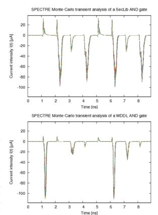
Figure 9: Monte-Carlo simulation results for SecLib (top) and WDDL (bottom).
