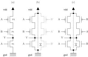
Figure 2: Transistor-level schematic of a SNOR gate.
