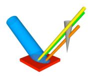
Figure 5: schematic illustration describing how the diffracted X-ray beam can imping on the AFM tip, resulting in figure 3b.
