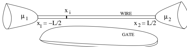
Figure 1: A quantum wire with an impurity, adiabatically coupled to metallic leads and to a metallic gate. The leads are held at different chemical potentials \mu_1 = eV_1 and \mu_2 = eV_2 .
