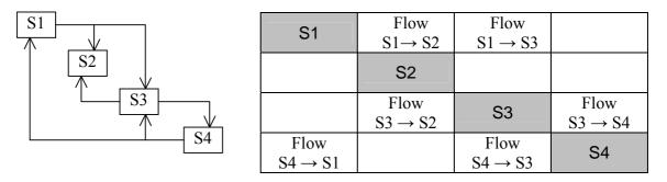
Figure 1. Coupled systems and the resulting coupling matrix.
