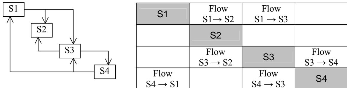
Figure 1. Coupled systems and the resulting coupling matrix.
