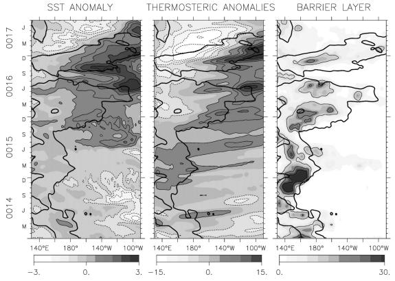
FIG. 3. Time-longitude sections averaged between 2°N and 2°S of SST anomalies, thermosteric anomalies referenced to 500 dbar, and barrier layer thickness simulated by the coupled model during years 14 to 17. The thick black line represents the 28.5°C SST isotherm. The contour interval is set to 0.5°C, 3 dyn cm, and 10 m. Dashed contours correspond to negative values.
