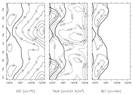
FIG. 2. Time–longitude sections averaged between 2°N and 2°S of the seasonal cycle simulated by the coupled model for SST, surface zonal wind stress, and barrier layer thickness. The thick black line represents the 28.5°C SST isotherm. The contour interval is set to 1°C, 0.01 N m<sup>-2</sup>, and 10 m.
