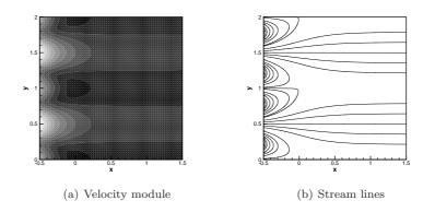
FIGURE 2. Plot of Kovasznay's solution for k = 1 and mesh 5.
