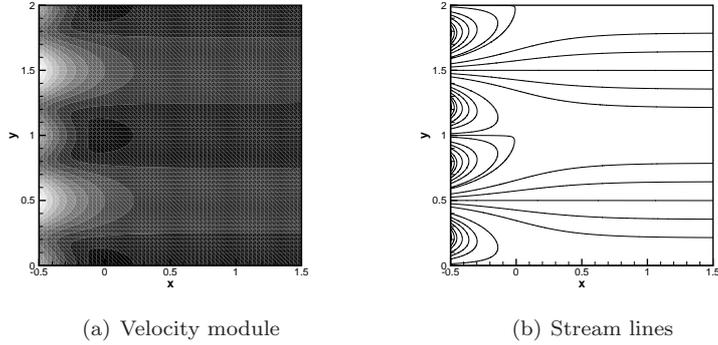
FIGURE 2. Plot of Kovaszny's solution for  $k = 1$  and mesh 5.
