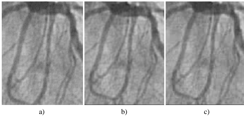
Figure 7.8. a) Original enhanced cardiac angiogram; b) pre-enhanced Full-Frame DCT coded image ( CR=12,8:1 ); c) enhanced JPEG coded image ( CR=12,8:1 ); from [BER 95]
