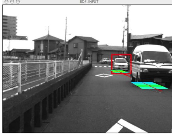
**Figure 2.** Example of BOF output using a computer vision car detector as input (red boxes). The images are provided by a camera mounted on the moving ego-vehicle. The BOF output is projected back on the image. It represents a grid of occupancy probability (blue-to-red mapped color) and the mean velocity (red arrows) estimates.
