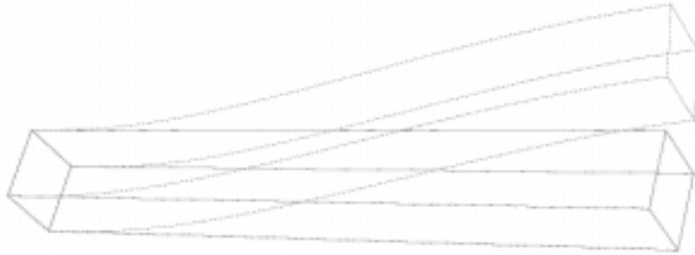
Figure 4.1: Buckling of the beam
