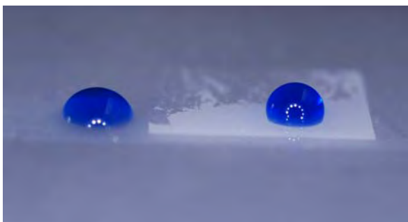
Figure 11. Different wetting behaviors due to the surface sub-micro structuring of the polymer substrate: honeycomb with wall thickness of 400nm (right), honeycomb with wall thickness of 1000nm (left).
