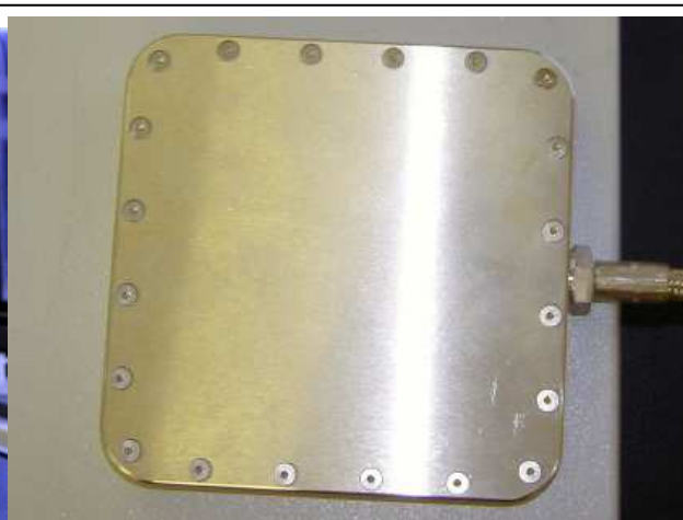
Fig. 2 Megasonic transducer of 4 by 4 inch active area
