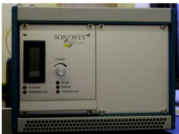
Fig. 1 Megasonic generator. 500 W Electrical power at 1MHz
