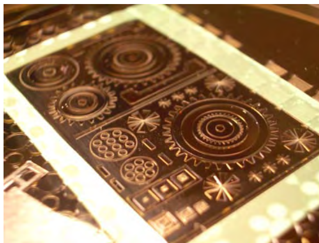
Fig.1. SU-8 photoresist mould on the conductive silicon wafer
