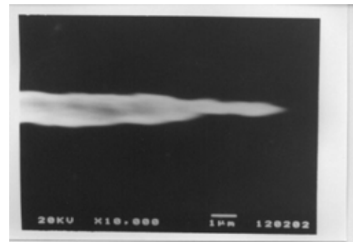
Fig.7 SEM photo of a micro probe by electrolysis. Dimension of micro probe with a tip of about 20nm. The machined current is 0.2mA, Voltage is 10V. The machine time is about 20min. The diameter before machining was 20µm.
