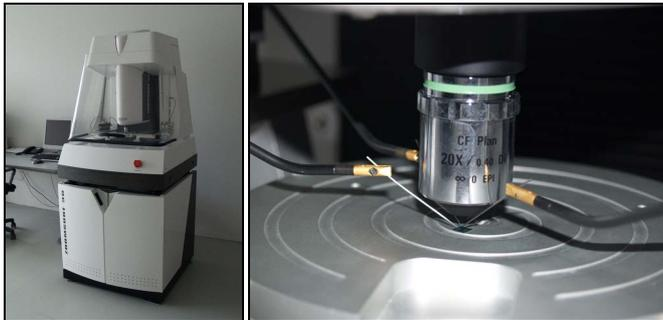
Fig. 3. Interferometric microscope Fogale ZoomSurf 3D (a) and the 20x Nikon objective (b).
