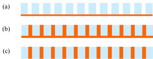
Fig. 2. Through-via filling after wafer thinning [10]: (a) Thinning / via formation/seed deposition; (b) Via filling; (c) Seed removal
