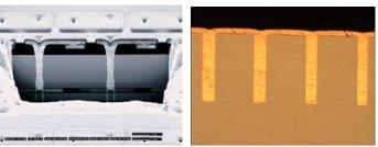
Figure 4: Solid filled vias a)W-CVD (courtesy IZM), b) Cu-ED (courtesy NEXX)
