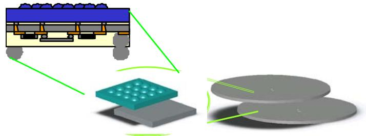
Figure 11: Hybrid integration of additional circuitry on the backside of a TSV enabled camera system
