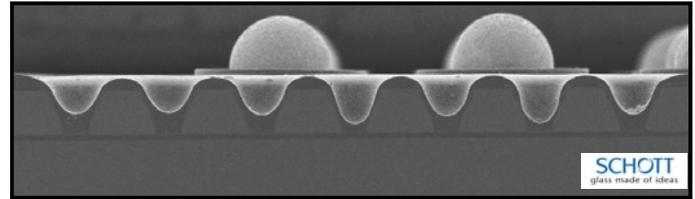
Figure 9: 3D TSV used for a camera chip in CSP format (courtesy SCHOTT)
