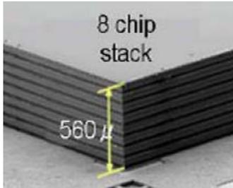
Figure 6: 3D Chip Stack using TSV's (courtesy Yole)
