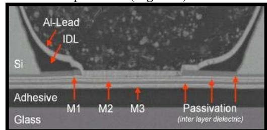
Figure 5: Thin film via contact (courtesy SCHOTT)
