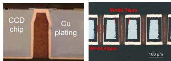
Figure 2: Blind TSV via with side wall copper fill (courtesy University of Arkansas), laser drilled through via with side wall fill based on laminate dielectric <sup>7/</sup>
