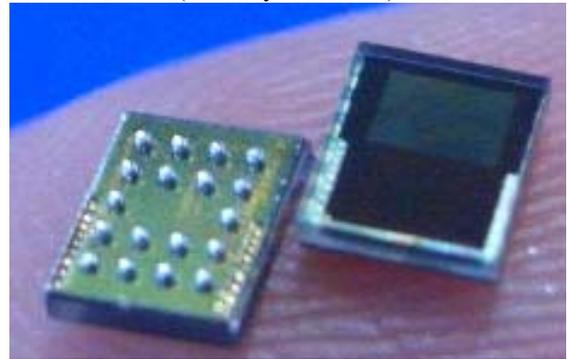
Figure 10: True wafer level CSP opto package (courtesy SCHOTT)
