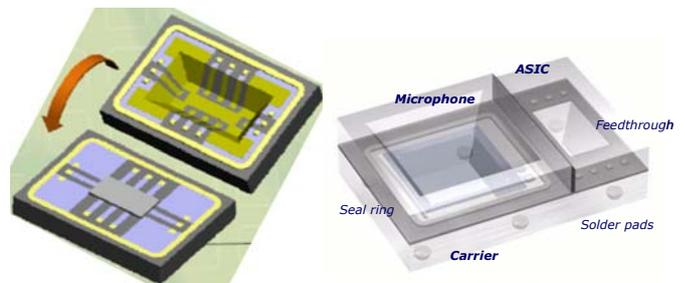
Figure 1: Routed via concepts through KOH etched holes for a) RF (courtesy Hymite) and b) MEMS systems (courtesy Sonion MEMS)
