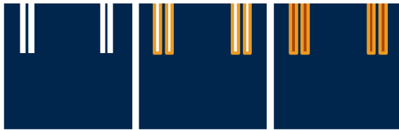
Fig. 2 : “Via first prior to FEOL” From left to right: D.R.I.E., Oxidation, Poly-Si refilling
