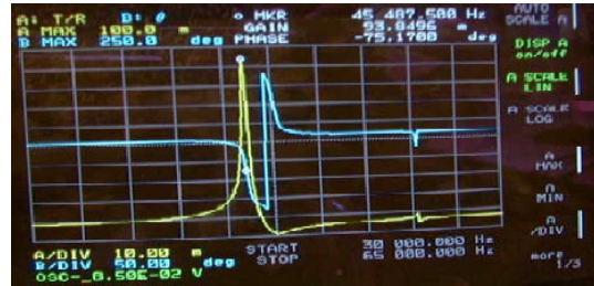
Fig. 6: Gain (0.093) and phase of a beam micro transformer using an uniform AlN film on the primary (input) and secondary (output) electrodes
