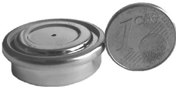
Fig. 13. Button cell hydrogen generator, size 3.5 cm 3 .
