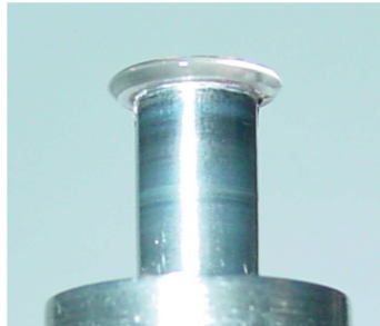
FIG. 2: MgF 2 optical resonator with 5.2 mm diameter on metal holder
