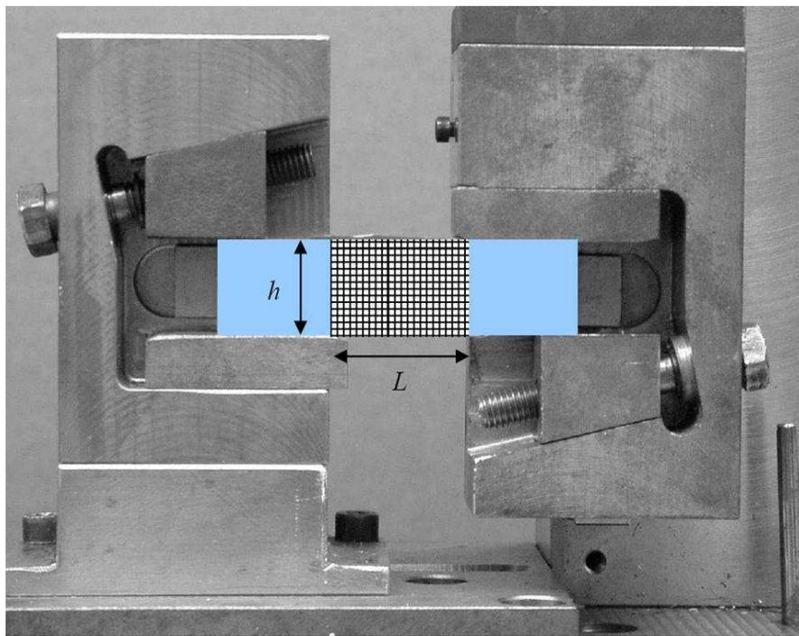
Figure 10: Shear-flexural test fixture with a schematic coupon.
