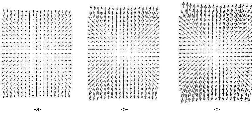
Figure 13: Biaxial test of a composite: measured displacement fields when  $F_1 = F_2 = 5\text{kN}$  (a),  $7\text{ kN}$  (b) and  $9\text{ kN}$  (c), with a magnification factor of 30. The failure load level is  $11.1\text{ kN}$ .
