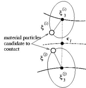
*Fig. 4.* Determination of material particles contact elements
