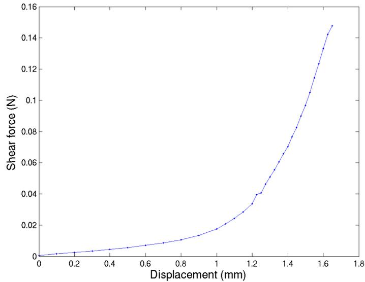
Fig. 13. Loading curve for the shear test
