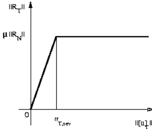
Fig. 7. Representation of the regularized friction model
