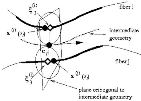
*Fig. 3.* Determination of cross-sections candidates to contact
