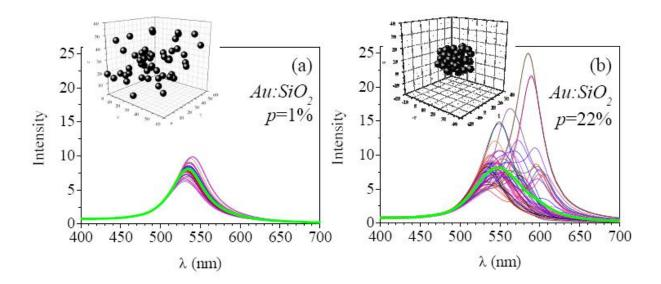
Figure 1. Relative local field intensity averaged in each particle,  $|f_{\ell}(\lambda)|^2$  (thin colored curves), and mean value in the whole sample corrected from edge effects (thick green curve) for a random distribution (insert) of 53 gold nanoparticles (2 nm radius) in a SiO<sub>2</sub> matrix, with metal concentration 1% (a) and 22% (b).
