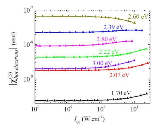
Figure 9. Variation of  $|\chi^{(3)}_{hot electrons}|$  with incident pulse peak intensity (pulse duration: 2 ps) and at selected photon energies in the virtual Au:SiO<sub>2</sub> thin film corresponding to Fig. 5.
