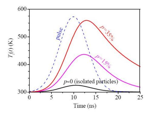
Figure 2. Temperature dynamics of gold nanoparticles ( $R_p = 1.3$  nm) in silica under pulsed laser excitation (pulsewidth: 7.5 ns, absorbed peak power:  $5 \times 10^{17}$  W m<sup>-3</sup>) for three metal concentrations. The pulse profile is reported in blue (arbitrary units).
