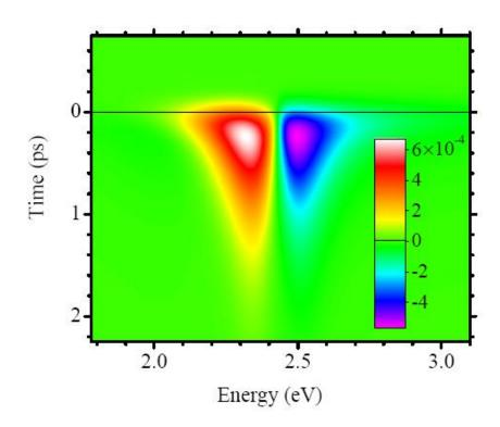
Figure 8. Spectral dispersion of the differential transmission (color level) as a function of pump-probe delay for the virtual thin  $Au:SiO_2$  film corresponding to Fig. 5, calculated by solving Boltzmann equation in the athermal regime. Pump photon energy: 1.55 eV; energy absorbed from the laser pulse:  $1.4 \times 10^{19}$  W m<sup>-3</sup>; pulse duration: 250 fs. The thin horizontal line at t=0 denotes the instant of pump-probe superimposition.
