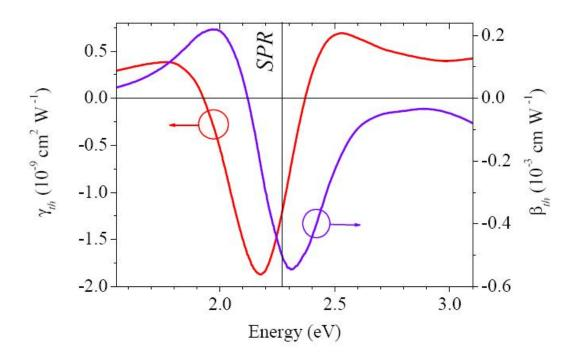
Figure 6. Calculated spectral dispersion of the thermal contribution to the nonlinear refraction (red) and absorption (violet) coefficients of the virtual thin Au:SiO<sub>2</sub> film under 7.5 ns laser pulses.
