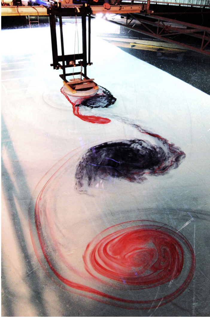
Fig. 5. A front view of a dye experiment for Ro \simeq 1 , Re \simeq 10,000 , and Bu \simeq 6.5 .
