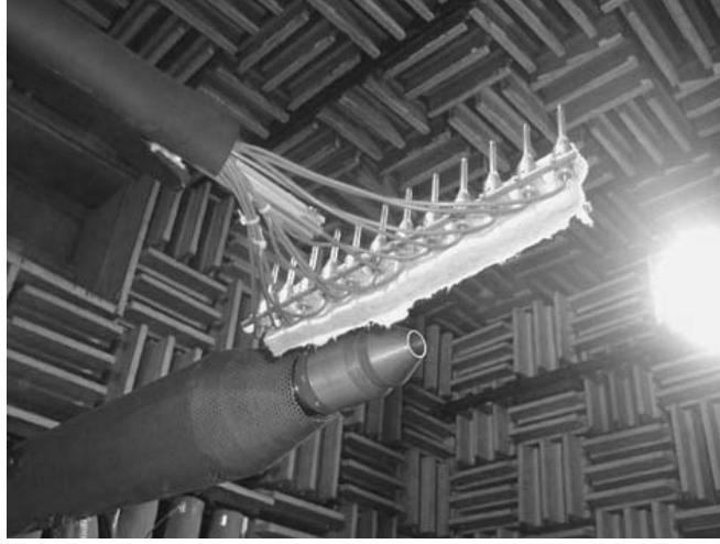
Figure 1: Experimental set-up used for the investigation of near-field jet noise.
