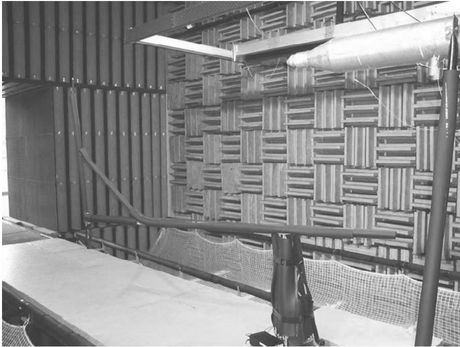
Figure 2: Experimental set-up used for the investigation of far-field jet noise.
