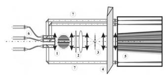
Fig. 1. Scheme of the AMBER configuration: (1) multiaxial beam combiner; (2) cylindrical optics; (3) anamorphosed focal image with fringes; (4) "long slit spectrograph"; (5) dispersed fringes on 2D detector; (6) spatial filter with single mode optical fibers; (7) photometric beams.
