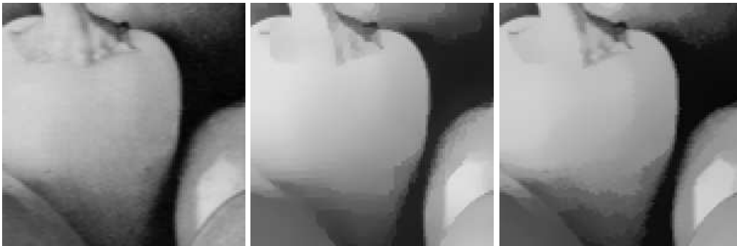
Fig. 1. Comparison between the neighborhood filter and the Perona-Malik equation. Left: original image. Middle: Perona-Malik filtered image. Right: filtered image by the neighborhood filter. The filtered images are very similar and both share artificial contours and flat zones that have been created inside the homogeneous regions.
