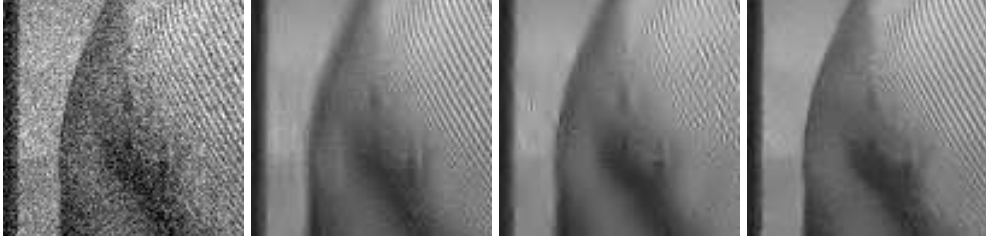
FIG. 6.9. Denoising experience on a natural image. From left to right and from top to bottom: noisy image (standard deviation 25), the DCT empirical Wiener filter, Hard TIWT and NL-means algorithm.
