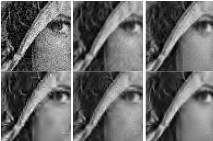
FIG. 3.2. Denoising experiment on a natural image. From left to right and from top to bottom: noisy image (standard deviation 20), Fourier Wiener filter (ideal filter), the DCT empirical Wiener filter, the wavelet hard thresholding, the soft wavelet thresholding and the translation invariant wavelet hard thresholding.
