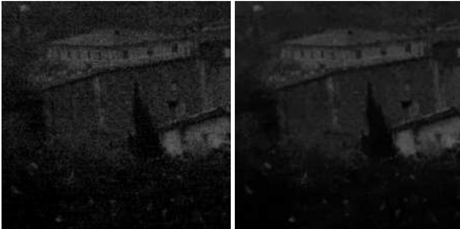
FIG. 6.12. Detail of Figure 6.11. Left: Original detail. Right: NL-means filtered detail.
