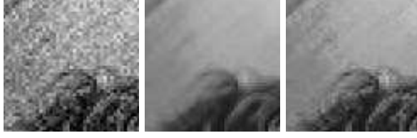
FIG. 5.7. Optimal correction experience. Left: Noisy image. Middle: NL-means solution. Right: NL-means corrected solution. The average with the noisy image makes the solution to be noisier, but details and fine structure are better preserved.
