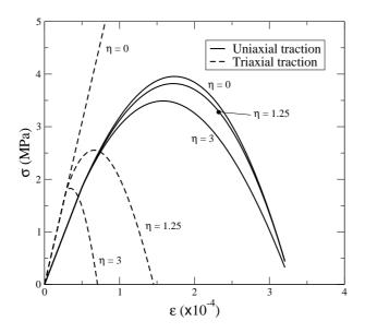
Figure 15. Effect of parameter  $\eta$  for uniaxial (continuous line) and triaxial (dashed line) tension tests  $(E = 37 \text{ GPa}, \nu = 0.2, \kappa_0 = 5 \times 10^{-5}, a = 3 \times 10^{-4} \text{ and } A = 5 \times 10^3).$
