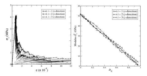
Figure 8. Stress-strain responses for the three directions during tri-tension (left), and evolution of stiffnesses  $\tilde{E}_1, \tilde{E}_2, \tilde{E}_3$  (right).
