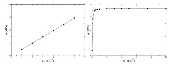
Figure 5. Evolution of tension peak stress versus model parameters  $\varepsilon_{cr}$  and  $\theta_{cr}$ .
