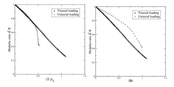
Figure 11. Evolution of  $\tilde{K}/K = 1/h(\mathbf{D})$  versus hydrostatic damage (left, in fact versus  $\sqrt{3}D_H$  for comparison) and versus the norm  $\|\mathbf{D}\|$  (right) for the 16-cube sample.
