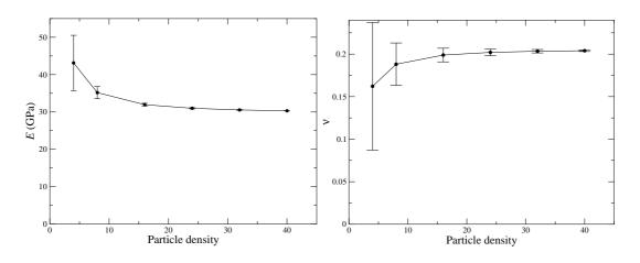
Figure 3. Convergence of elastic parameters with respect to particle density
