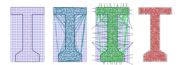
Figure 1. Successive steps of the mesh generation.
