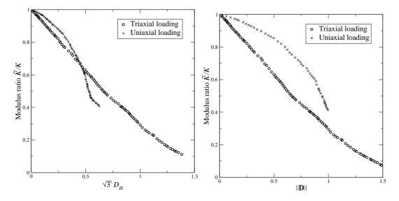
Figure 9. Evolution of  $\tilde{K}/K = 1/h(\mathbf{D})$  versus hydrostatic damage (left, in fact versus  $\sqrt{3}D_H$  for comparison) and versus the norm  $\|\mathbf{D}\|$  (right) for the 8-cube sample:  $h(\|\mathbf{D}\|)$  exhibits a loading dependency when  $h(D_H)$  is kept invariant and can be considered as intrinsic.
