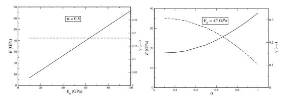
Figure 4. Evolution of elastic material parameters E and  $\nu$  versus beam parameters  $E_b$  and  $\alpha$ .
