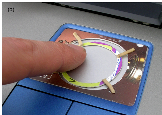
Figure 11: RubberEdge prototype device: (a) Schematic; (b) implementation.
