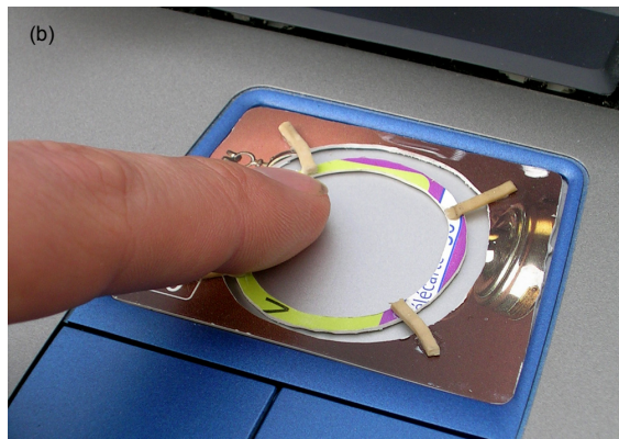
Figure 11: RubberEdge prototype device: (a) Schematic; (b) implementation.
